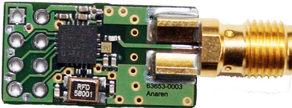
Figure 6: Anaren Solution with 0402 Matching Network
