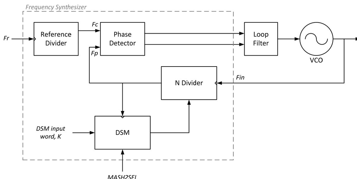
One of the consequences of the DSM is its generation of fractional spurs due to the accumulation of random phase errors. Delta-sigma noise shaping techniques are applied to fractional-N synthesizers to shift unwanted spurs outside the bandwidth of the loop filter. However, the valid divide ratio is further limited by the delta-sigma modulator due to variation of the instantaneous division ratio around the average correct division ratio.
