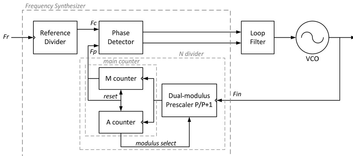
The main counter chain then divides the prescaler output by an integer derived from the settings in the M and A counters. Programming the M counter with the minimum allowed value of “1” will result in a minimum M counter divide ratio of “2”. Therefore, the output from the main counter chain ( $F_P$ ) is related to the VCO frequency ( $F_{IN}$ ) by:
