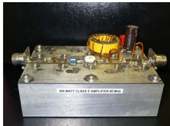
Figure 8. Prototype of class E amplifier
