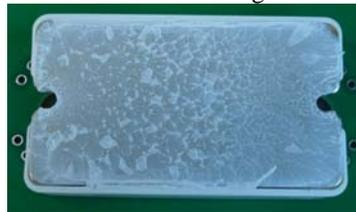
Picture 10: Grease on the module after disassembling
