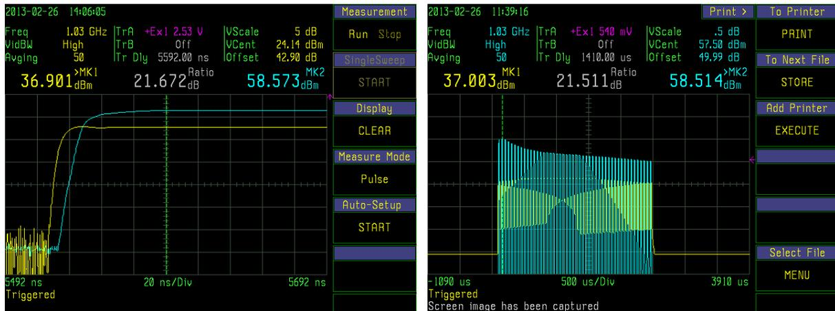
**Figure 7 – 1011GN-700ELM short pulse & ELM long pulse rise time performance**
