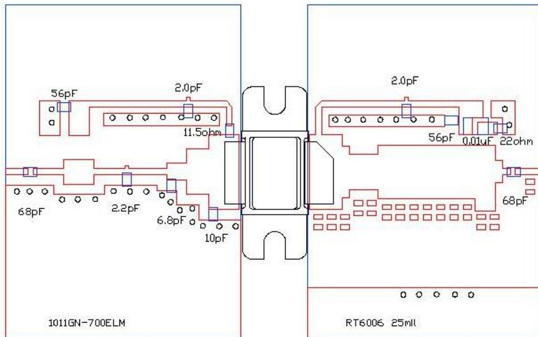
**Figure 5 – 1011GN-700ELM Evaluation Test Fixture RF Circuits**
