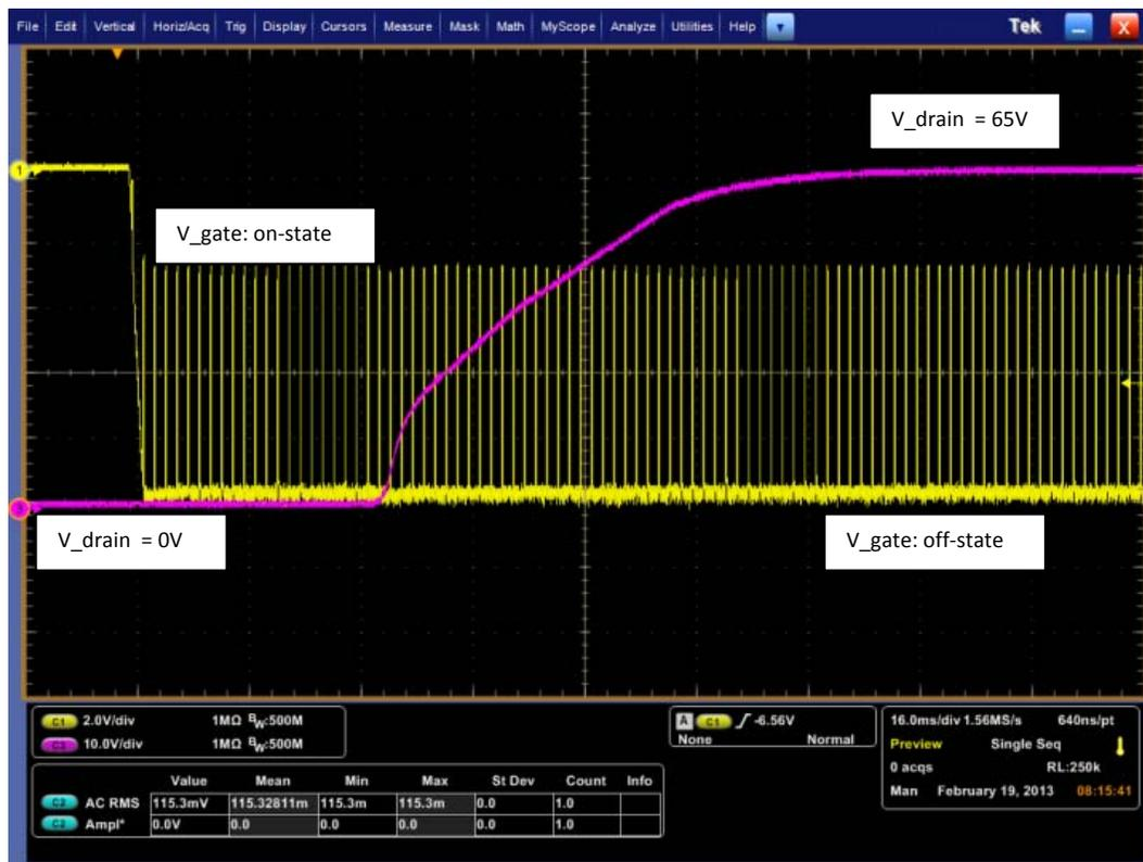
**Figure 4 – Typical pulsed GaN RF power transistor  $V_{dd}$  drain bias sequencing timing**
