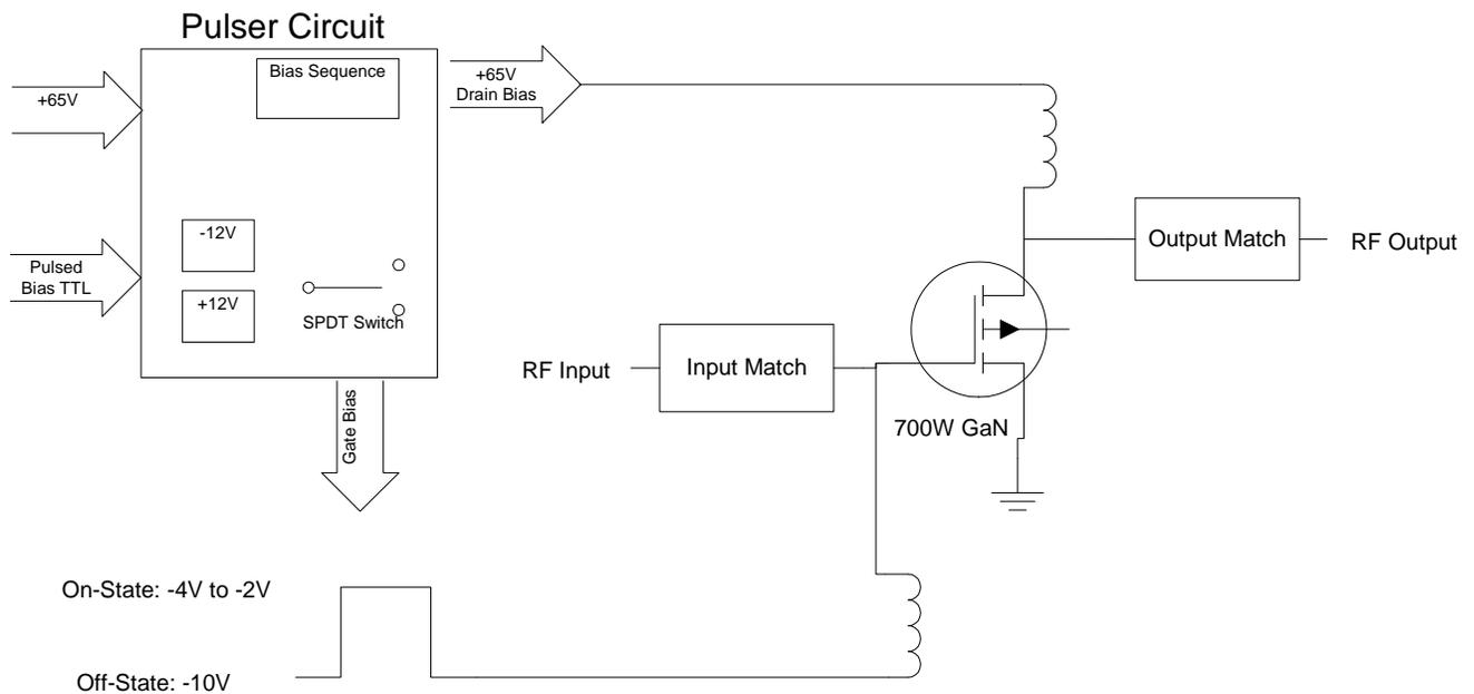
**Figure 1 – Typical Microsemi GaN RF power transistor evaluation test circuit block diagram**
