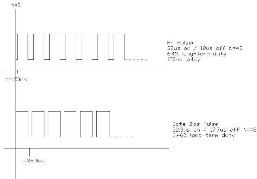
**Figure 3 – Typical Mode-S ELM RF Pulsing**
