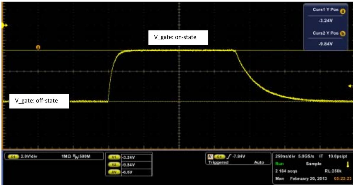
**Figure 2 – Typical negative Vgs gate OFF (-12V) to ON (-3.2V) pulsing**
