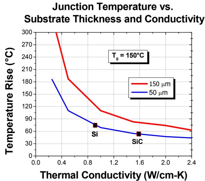
**Figure 4: Temperature rise of GaN devices show reduced sensitivity to substrate thermal conductivity as die thickness is reduced. Thus, the benefit of thermal conductivity of SiC when compared to Si diminishes as die thickness is reduced.**
