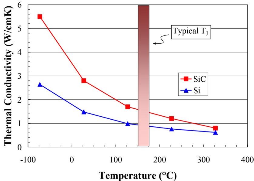
Figure 3. Thermal conductivity over temperature for Si and SiC <sup>16</sup>.
