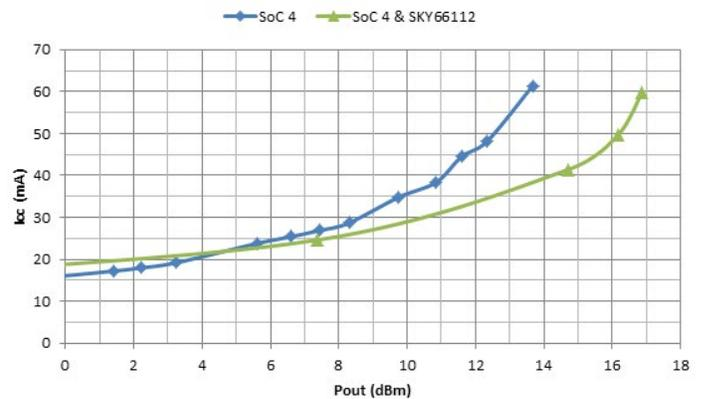
Figure 2. Pout vs. Icc with DC-DC Enabled
