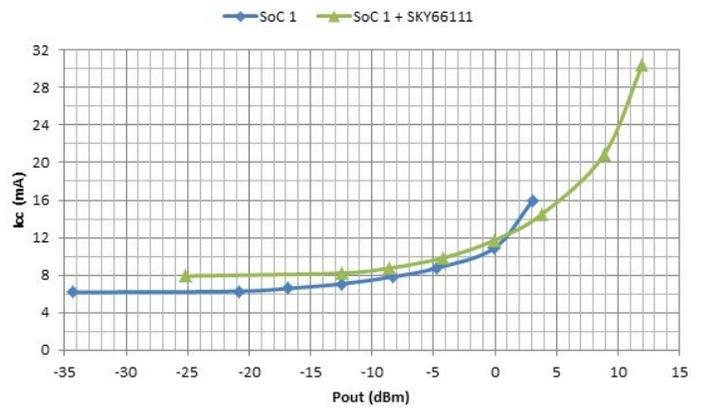
Figure 7. Transmission power vs. total system current.
