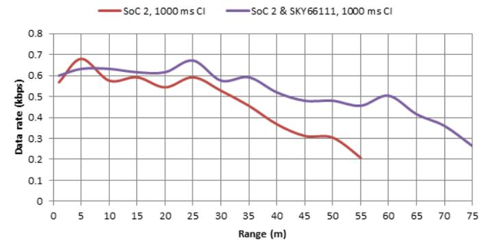
Figure 9. Data Rate vs. Range, Low Data Rate
