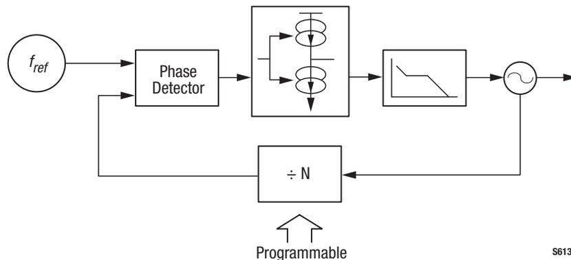
**Figure 1. Basic Integer-N Synthesizer Architecture**
