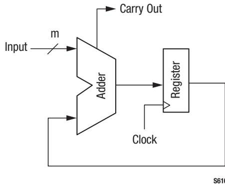
Figure 4. Design of a Simple Digital Phase Accumulator
