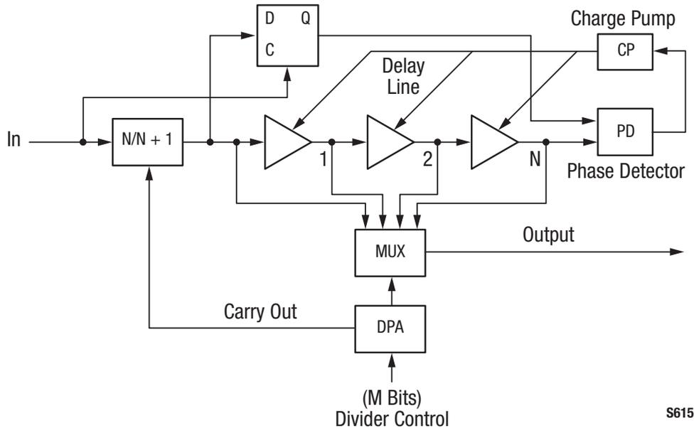
Figure 3. Example of Fractional-N Divider Implementation
