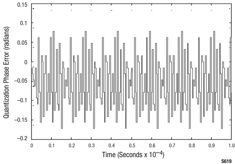
**Figure 7. Quantization Phase Error for a 4<sup>th</sup> Order  $\Delta\Sigma$  Modulator**
