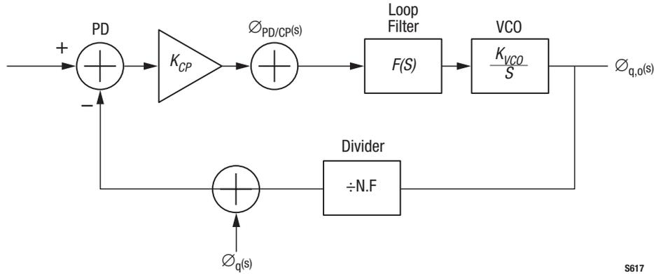
Figure 5. A Linearized Phase-Domain Model of a PLL With Quantization Noise Source
