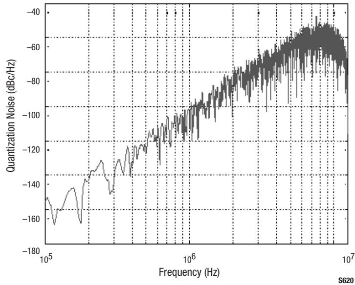
**Figure 8. Quantization Phase Noise Spectrum Corresponding to the Waveform in Figure 7**
