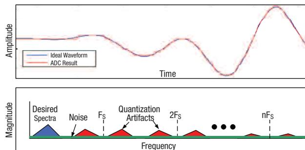
**Figure 3. Time and Frequency Domain Representations of a Quantized Analog Waveform—A Unique Reconstruction Filter Setting is Required for Each Sampling Rate**
