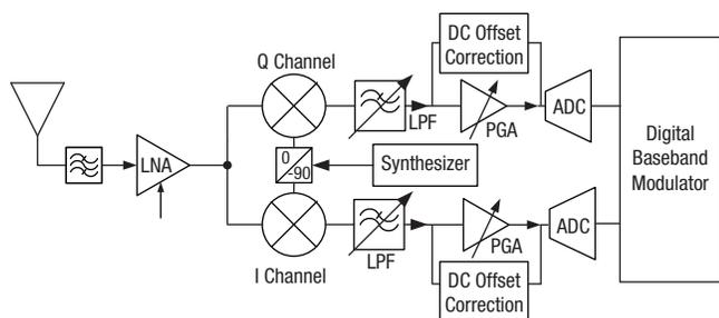
**Figure 4. A Flexible Channel Direct Conversion Receiver**
