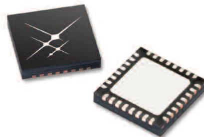
**Figure 1. The SKY73201-364LF (Single) and SKY73202-364LF (Dual) 6th Order Programmable Butterworth Filters In a 32-lead, 5 x 5 mm MLP Package**
