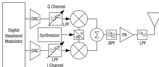
**Figure 2. A Typical Direct Conversion Transmitter Chain with Programmable Reconstruction Filters**
