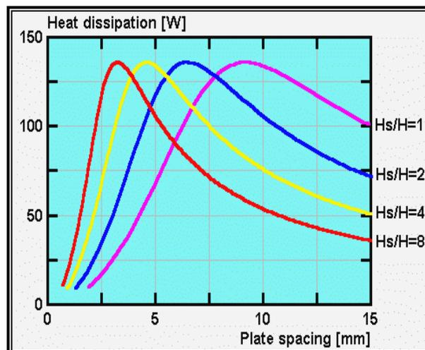
Figure 3 shows a typical result of a calculation that involves several Chimney-to-Plate Height Ratios, (Hs/H). The main impact of this parameter is that it tends to decrease the optimum plate spacing. The total heat dissipation is, as expected, the same for all cases.
