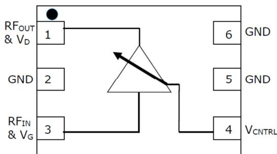
**Figure 3. MAAM-011100 VGA Schematic**
