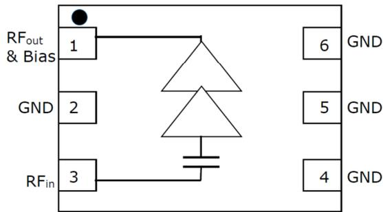
**Figure 1. MAAM-011101 GPA Schematic**
